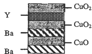
Figure 4. Unit structure of \text{YBa}_2\text{Cu}_3\text{O}_x
